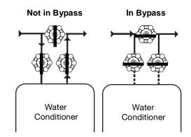
Figure 2 - Typical Globe Valve Bypass System
